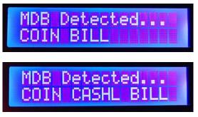
After finished the device detecting, then it enters the normal operation interface. Then it is possible to make payment through the payment device
