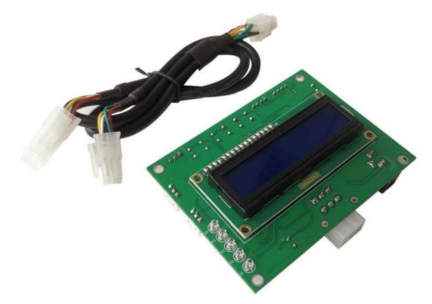
LCD panel on the front side for device information Five LED to show the device working status
